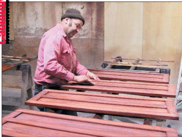
Van Dusartz Quality Woodworking does its own staining in a large, 40-by-60-foot spray booth, which is located in a separate building.
